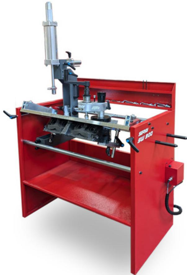
Multipurpose work station with easy access to fireface or camshaft side of the cylinder head.
