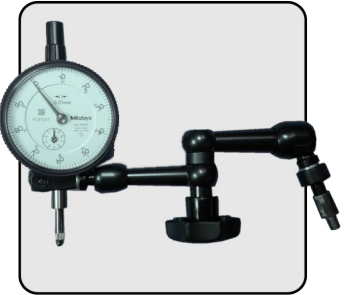
To machine the seats to the same depth position. Inch version.
