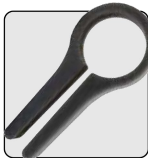
Tightening or lossening the spindle nut with the right strength.
