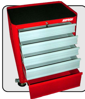
The Serdi tool cart allows stocking tool holders, tools, pilots, pads...used with the machines.
